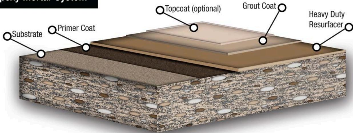
Epoxy Mortar Flooring System is a troweled, high strength concrete resurfacing material. It is used for environments requiring an industrial grade floor or when a concrete floor has sustained damage requiring a 3/16" to 1/4" surface restoration.
